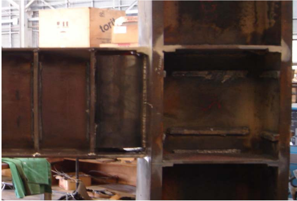
Figure 2.34: Specimen AISC-8 – Link-to-Column Connection Region – Frontside of Link
