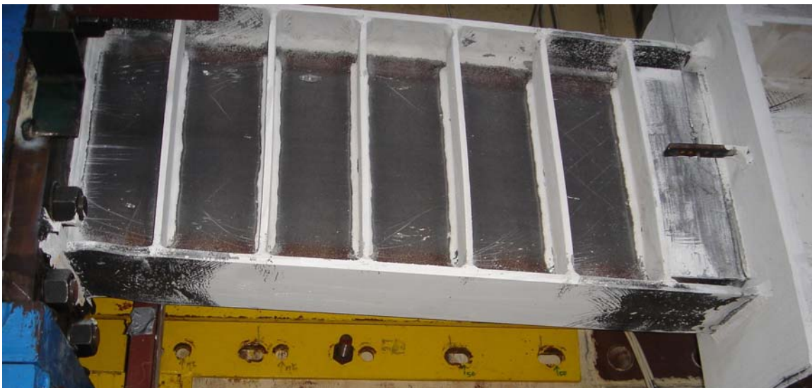
Figure 3.60: Location of Yielding at the Link Flanges after Failure of Specimen AISC-8 during Loading Cycle of \gamma = \pm 0.09 rad
