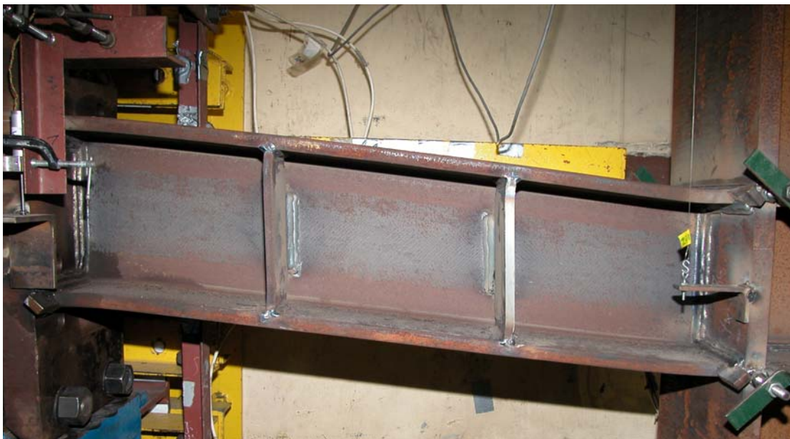
Figure 3.16: Specimen AISC-4 after Loading Cycle at \gamma = \pm 0.11 rad (Last full loading cycle prior failure)
