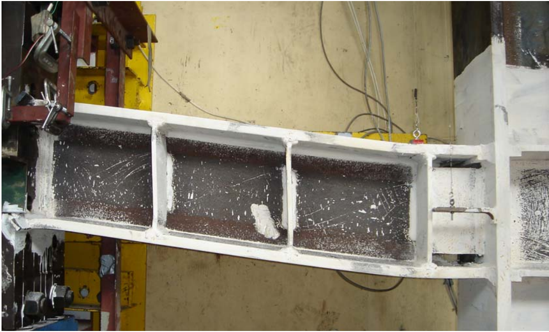
Figure 3.43: Specimen AISC-7 after loading cycle of \gamma = \pm 0.11 rad (Last full loading cycle prior to failure)
