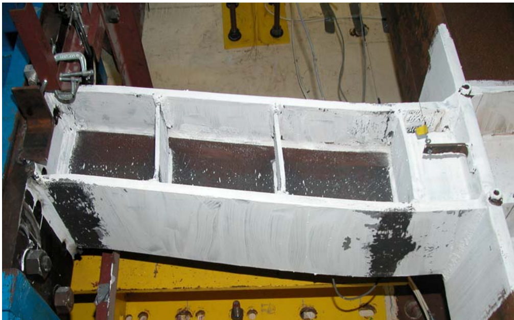
Figure 3.36: Specimen AISC-6 – Yielding confined in the Unreinforced portion (Last full loading cycle prior to failure)
