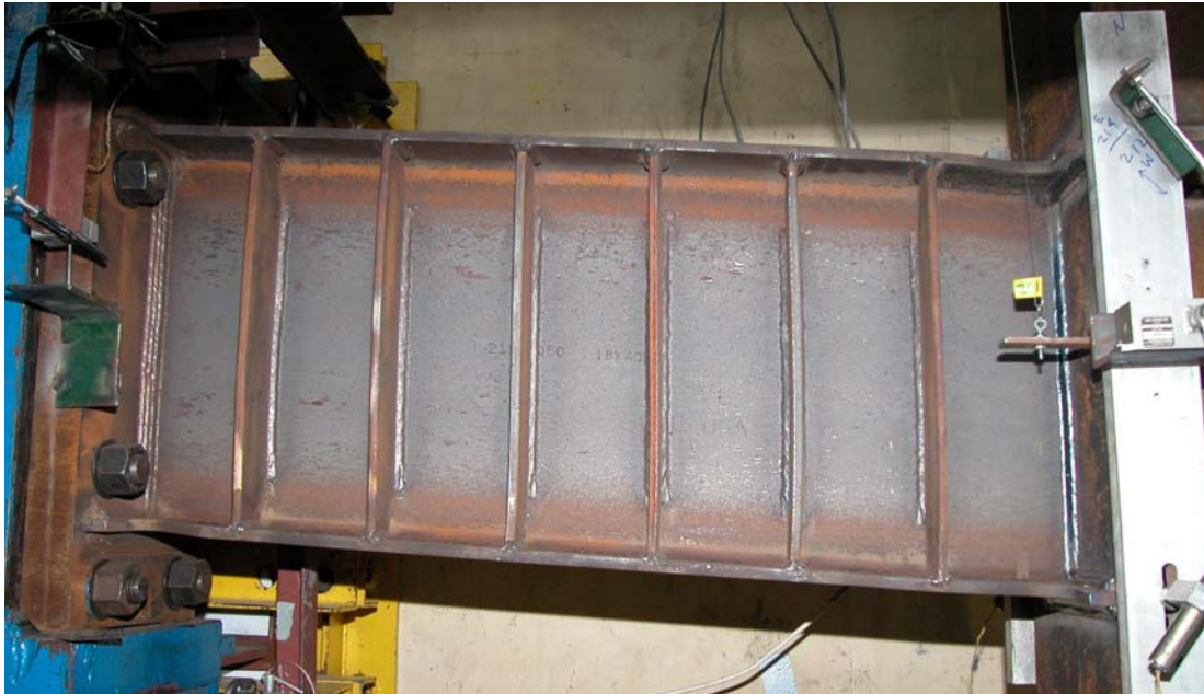
Figure 3.11: Failure of Specimen AISC-3 during loading cycle at \gamma = + 0.11 rad
