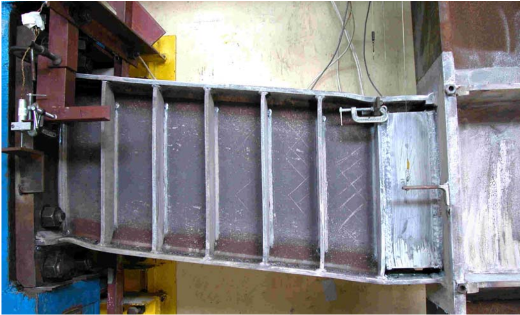
Figure 3.25: Specimen AISC-5 after First Loading Cycle at \gamma = + 0.11 / -0.13 rad (Last full loading cycle prior to failure)
