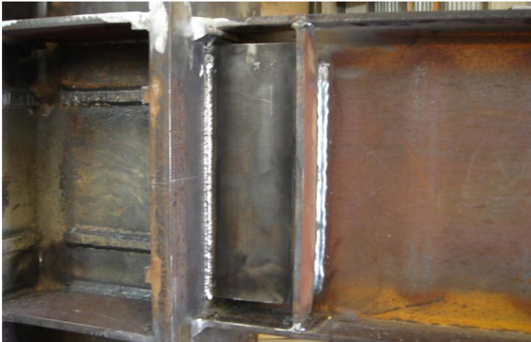
Figure 2.35: Specimen AISC-8 after Completion of Fabrication – Backside of Link
