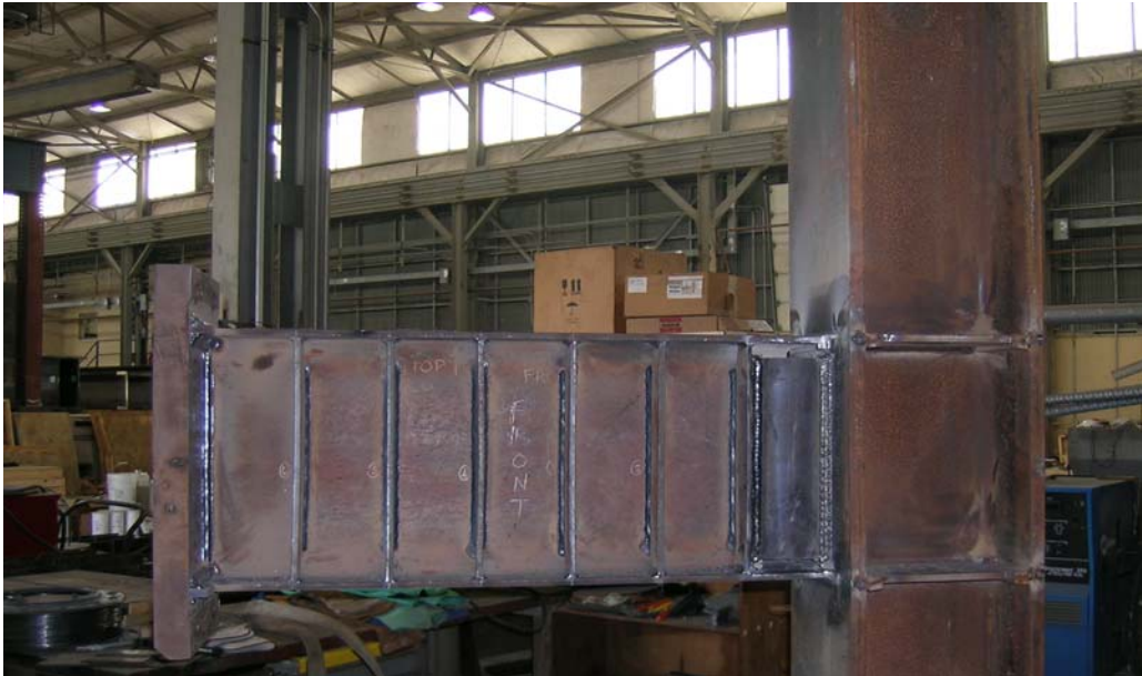
Figure 2.30: Overall View of Specimen AISC-5 after Completion of Fabrication
