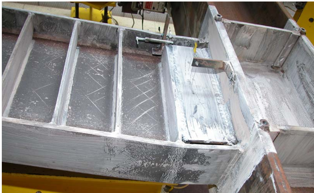
Figure 3.26: Yielding restricted primarily away from the link-to-column connection (Last full loading cycle prior to failure)
