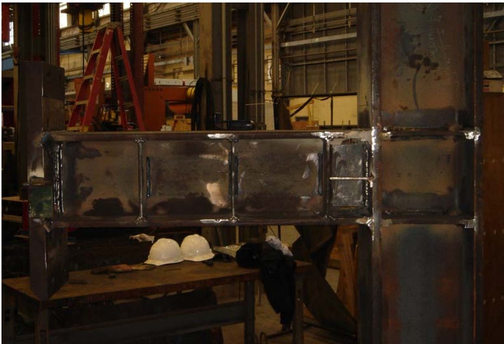
Figure 2.43: Overall View of Specimen AISC-7 after Completion of Fabrication
