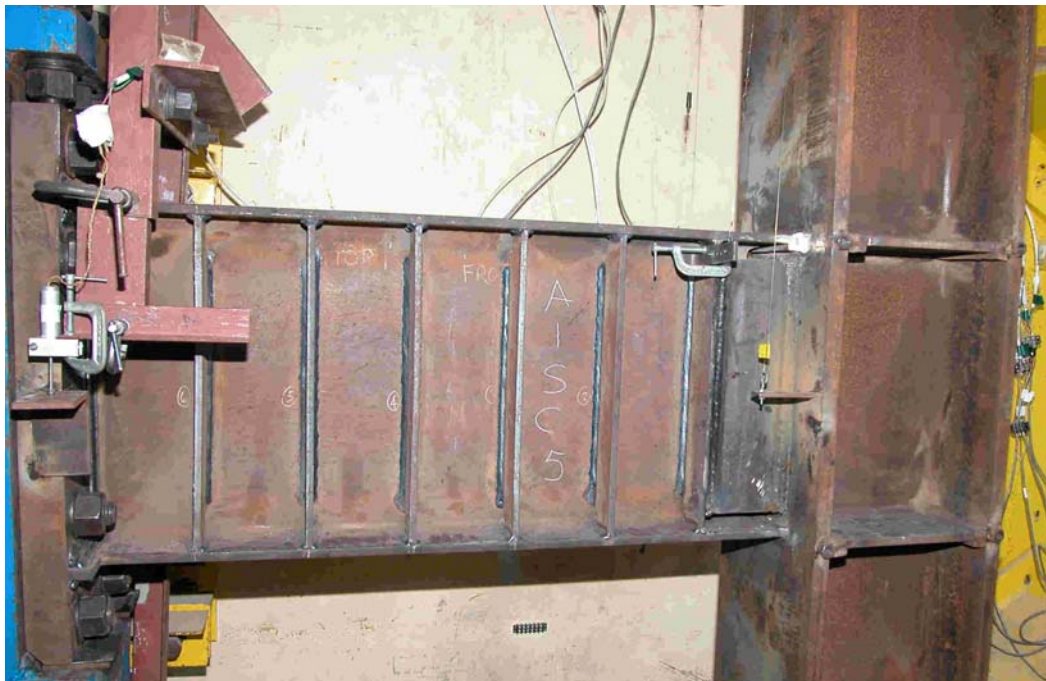
Figure 3.24: Specimen AISC-5 prior to Testing and Whitewash
