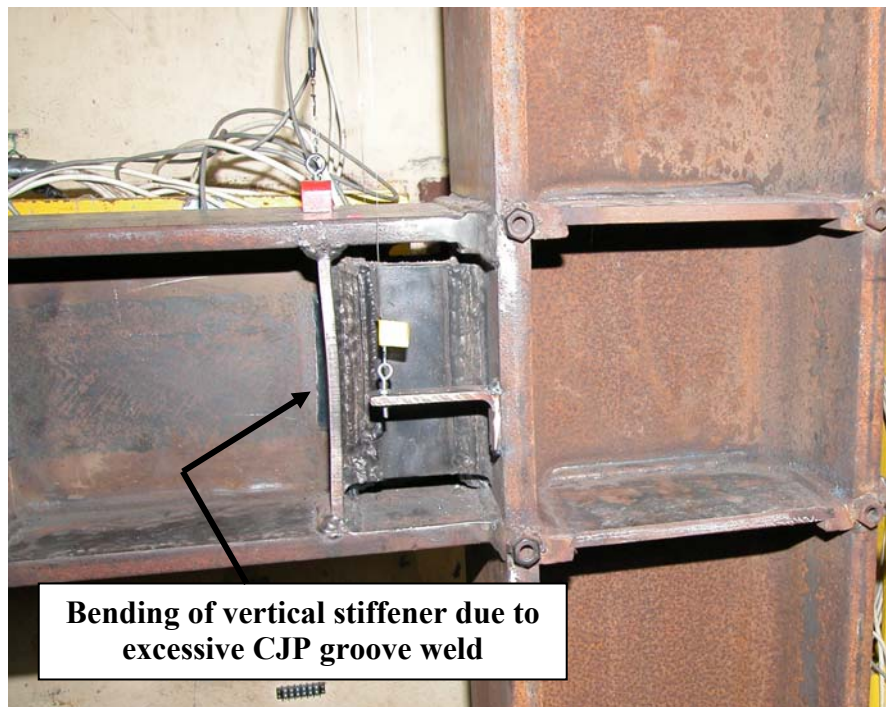
Figure 3.34: Specimen AISC-6 – Link-to-Column Connection
