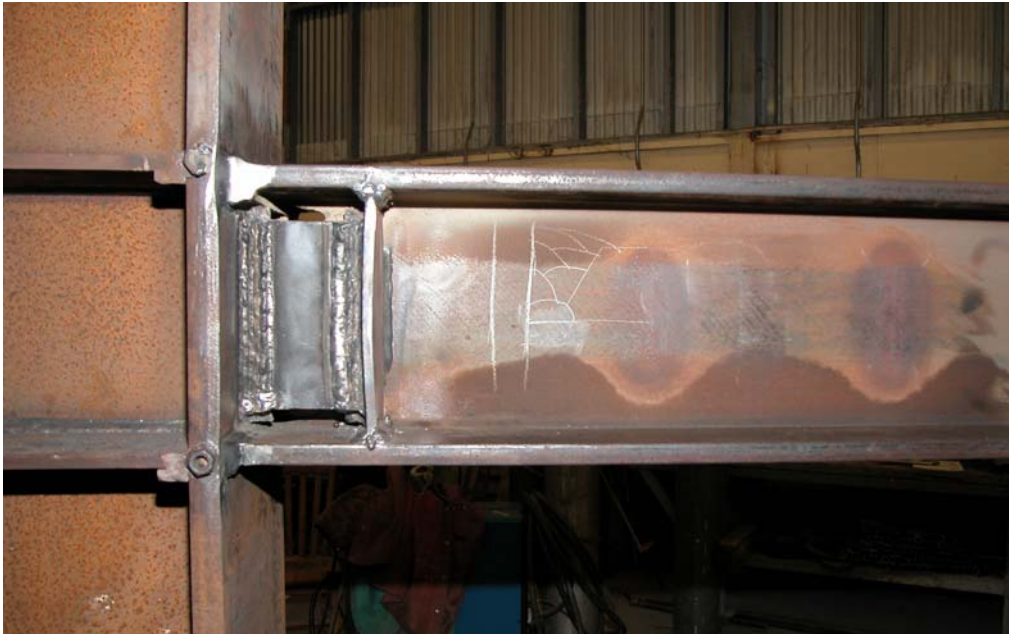
Figure 2.42: Specimen AISC-6 after Completion of Fabrication – Backside of Link
