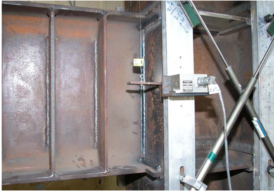
Figure 2.12: Link-to-Column connection detail for Specimens AISC 1 to 3
