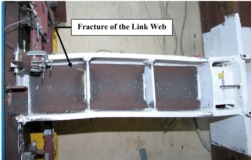
Figure 3.37: Failure of Specimen AISC-6 during 2 nd loading cycle of \gamma=+0.12/-0.13 rad (Failure by fracture of the link web adjacent to vertical stiffener)
