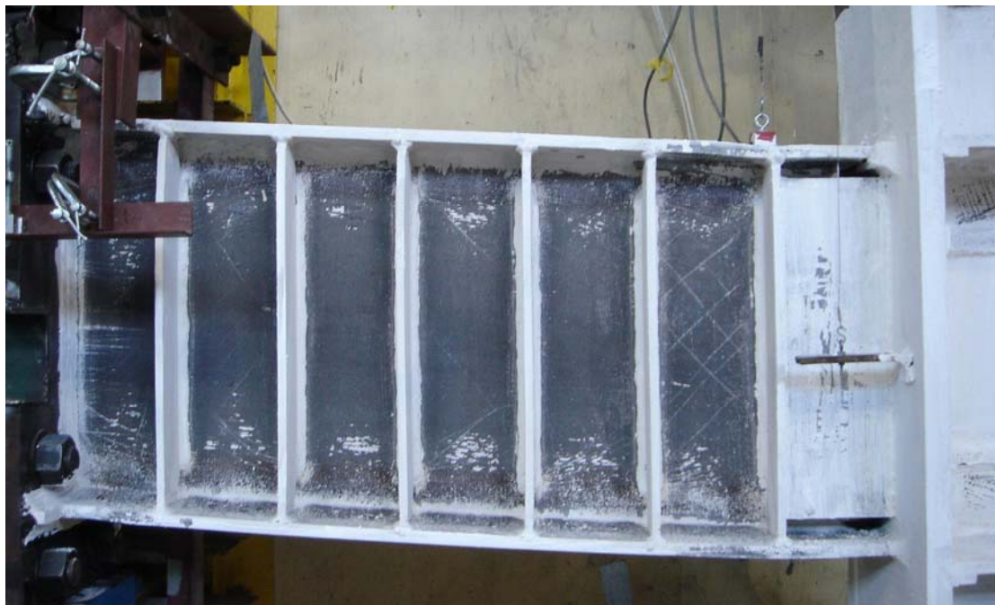
Figure 3.54: Specimen AISC-8 after Loading Cycle of \gamma = \pm 0.07 rad (Last full loading cycle prior to failure)
